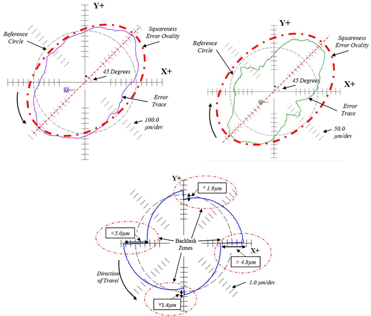
**Fig. 3.** (top left) Control ballbar result trace in CCW direction; (top right) control ballbar result trace in CW direction showing squareness error identification as no orientation change from CCW trace; (bottom) simulated pure backlash for demonstration of effect.
