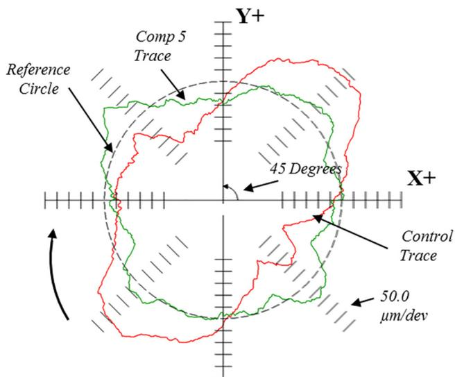
**Fig. 4.** Comparison of uncompensated ballbar test trace (red) versus compensated ballbar test trace (green) showing the improvement in contouring and accuracy performance.
