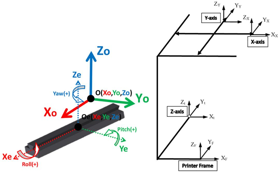
Fig. 2. (left) Visualisation of a translational axis: 6 kinematic errors, 3 translation, and 3 rotational; (right) kinematic configuration of Ultimaker Original showing the parallel chain configuration.
