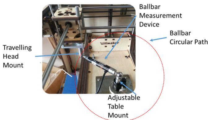
Fig. 1. Ballbar setup on Ultimaker Original with modifications to printer.
